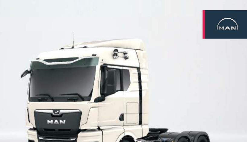
Cabina GM: ANCHA TECHO ALTO (ancha, larga, altura media), dos literas
