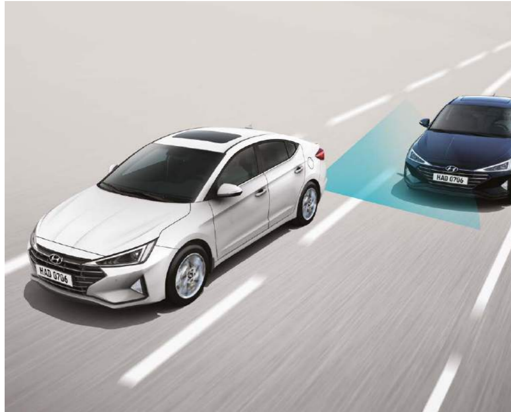
Blind-Spot Collision Warning (BCW) Reflexive radar sensors in the rear bumper warn the driver of approaching vehicles that aren't visible.
